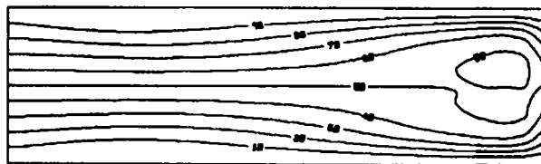
Figure 5. Problem 2—solution for \psi - v streamfunction (percentages of maximum streamfunction)
